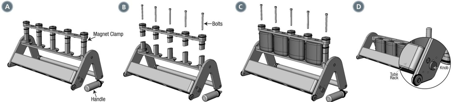
(A) EasySep™ Multistand with the handle off and magnet holder inverted.
