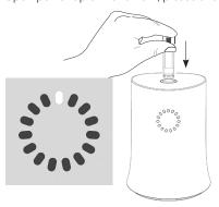
Instrument is warmed up and in "ready" state. Insert a clean, tightly capped frozen 1.8 - 2.0 mL cryogenic vial (below -70°C) containing up to 1.8 mL volume into the opening on the top of the instrument.
