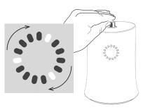
Push the top of the vial down gently until the instrument emits a deep dual tone. The vial will now remain in a depressed position.
