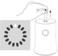
Remove vial immediately and for a few seconds, manually agitate the vial gently from side to side to equilibrate the liquid temperature until no ice can be seen within the vial. Begin downstream protocol.
