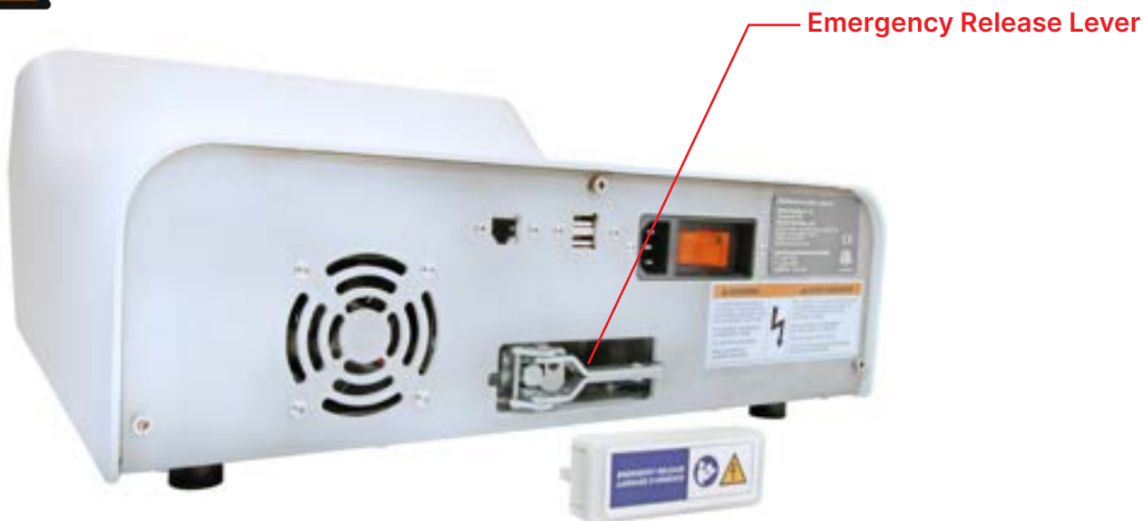
Figure C: Back of the ThawSTAR® CB with Emergency Release Cover Removed
