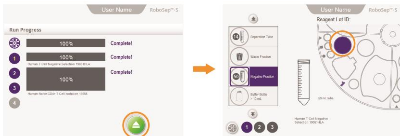
Figure 24. Collecting Isolated Cells at the End of a Protocol Run. The desired isolated cells are in the tube highlighted in color in quadrant #1 of the Unloading screen.
