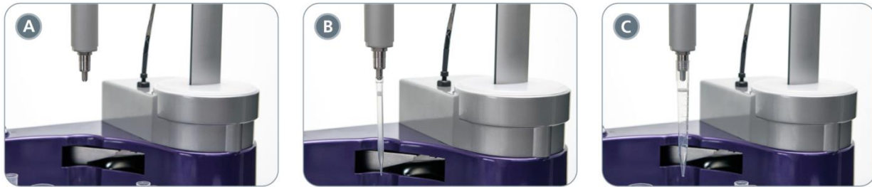
Figure 4. Tip Head on the Robotic Arm. The tip head (A) before picking up a tip and after picking up a disposable (B) 1 mL tip and (C) 5 mL tip.
