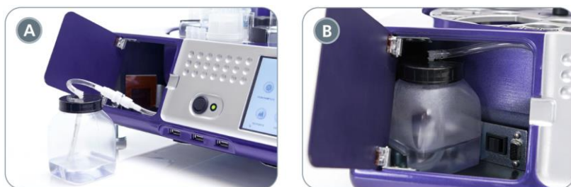
Figure 15. Hydraulic System. The hydraulic bottle and quick release (A) outside and (B) inside of the instrument.
