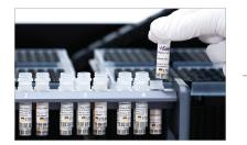
Select protocol. Load sample, EasySep™ reagents, buffer, and tips.
